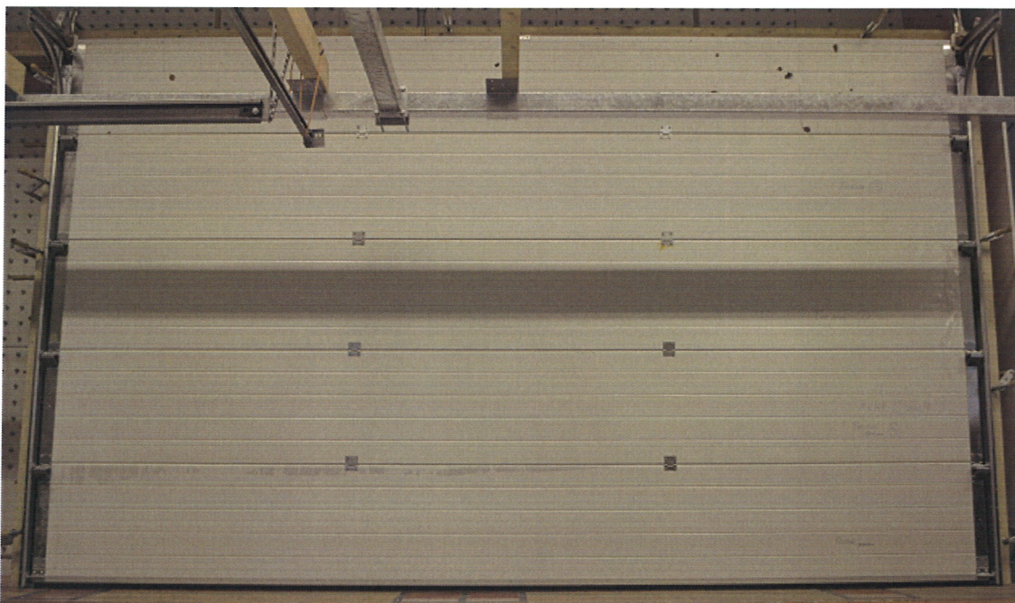
Figure 1. Door type DOCO SFR Tecsedo, mounted in the test rig, as seen from inside.
